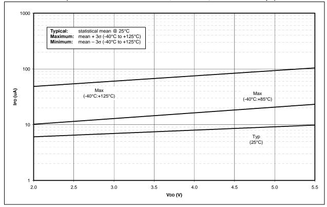
FIGURE 27-16: TYPICAL AND MAXIMUM Alwdt vs. Vdd OVER TEMPERATURE (WDT ENABLED)
