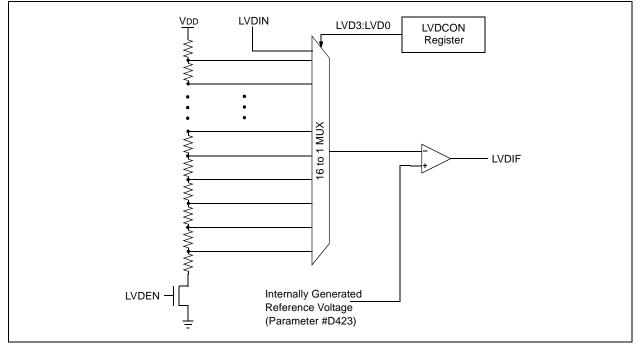
The LVD module has an additional feature that allows the user to supply the trip voltage to the module from an external source. This mode is enabled when bits LVDL3:LVDL0 are set to '1111'. In this state, the comparator input is multiplexed from the external input pin, LVDIN (Figure 22-3). This gives users flexibility because it allows them to configure the Low-Voltage Detect interrupt to occur at any voltage in the valid operating range.
