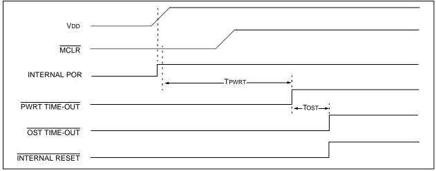
FIGURE 3-5: TIME-OUT SEQUENCE ON POWER-UP (MCLR NOT TIED TO VDD): CASE 2
