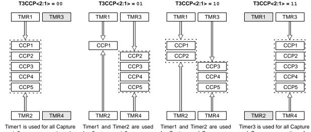
Timer1 is used for all Capture and Compare operations for all CCP modules. Timer2 is used for PWM operations for all CCP modules. Modules may share either timer resource as a common time base.
