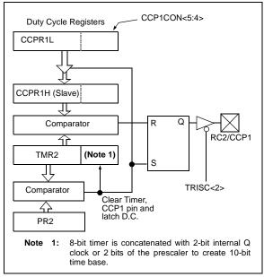
A PWM output (Figure 16-5) has a time base (period) and a time that the output stays high (duty cycle). The frequency of the PWM is the inverse of the period (1/period).
