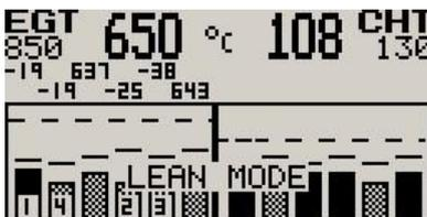
As the fuel mixture is slowly leaned past the point at which the temperature begins to drop (by more than 10°C/15°F), the absolute EGT temperatures will change to show the EGT reading relative to this peak. The sequential order as each cylinder peaks is also shown.
