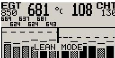
Fuel mixture should be adjusted once you have decided on a suitable cruise power setting (typically 70%). Press the Up/F1 key at the main display to enable the leaning mode. The "LEAN MODE" label is displayed at the bottom of the main display to clearly differentiate it from the normal operating mode.
