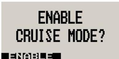
Once in the cruise, pressing the Down/F2 key will immediately enable Cruise Mode. The "CRUISE MODE" label is displayed at the bottom of the main display to clearly differentiate it from the normal operating mode. All EGT and CHT readings are immediately sampled as reference temperatures for the cruise.
