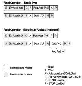
Figure 10. I<sup>2</sup>C Read Operation
