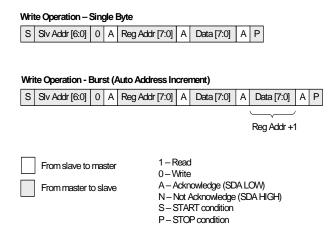
Figure 9. I<sup>2</sup>C Write Operation
