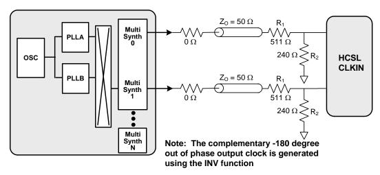
Figure 17. Si5351 Output is HCSL Compatible
