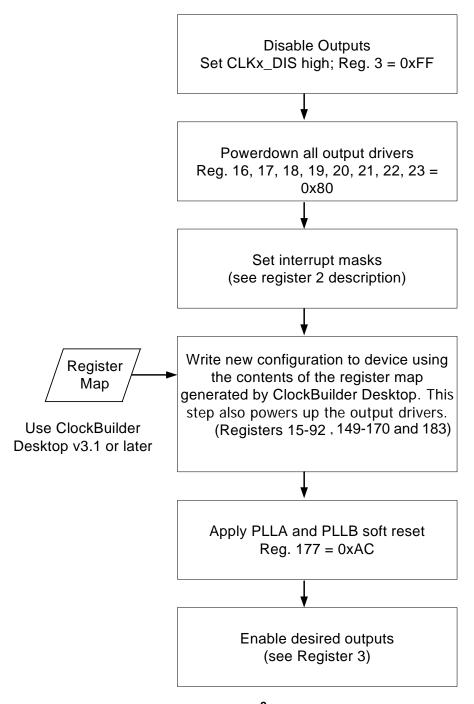
Figure 12. I<sup>2</sup>C Programming Procedure
