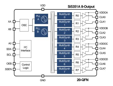
Figure 1. Block Diagrams of 3-Output and 8-Output Si5351A Devices
