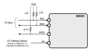
Figure 7. I<sup>2</sup>C and Control Signals
