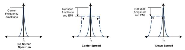
Figure 6. Available Spread Spectrum Profiles
