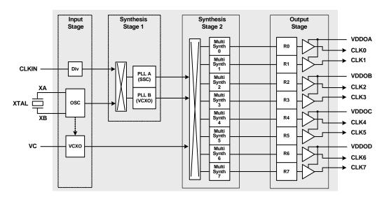
Figure 3. Si5351 Block Diagram
