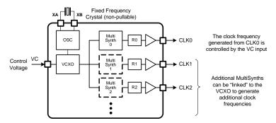
Figure 5. Using the Si5351 as a Multi-Output VCXO
