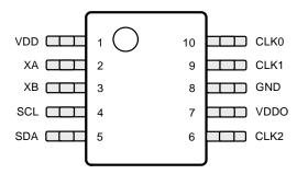
Figure 21. Si5351A 10-MSOP Top View
