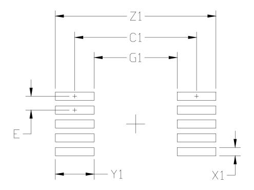
Figure 27. 10-Pin MSOP Land Pattern
