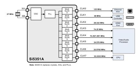
Figure 13. Using the Si5351A to Replace Multiple Crystals, Crystal Oscillators, and PLLs
