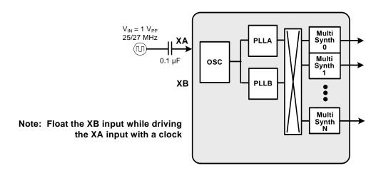
Figure 16. Si5351 Driven by a Clock Signal
