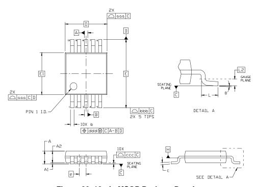
Figure 26. 10-pin MSOP Package Drawing
