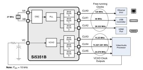
Figure 14. Using the Si5351B to Replace Crystals, Crystal Oscillators, VCXOs, and PLLs
