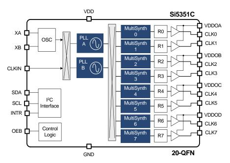
Figure 2. Block Diagrams of Si5351B and Si5351C 8-Output Devices
