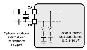
Figure 4. External XTAL with Optional Load Capacitors
