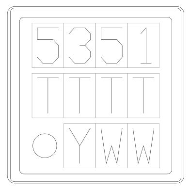
Figure 29. 10-Pin MSOP Top Marking
