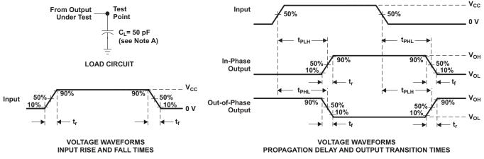
Figure 3. Load Circuit and Voltage Waveforms
