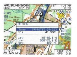
A waypoint, with the actual date and time automatically assigned as a name, has now been created with the present position and GPS altitude details.
