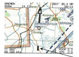
On takeoff or during flight, the position is shown by the circle and true-track by the arrow.
