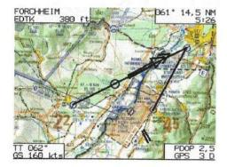
When the waypoint is reached, the black line in the area of the previous leg is deleted. The part of the leg still to go remains visible as a black line.
