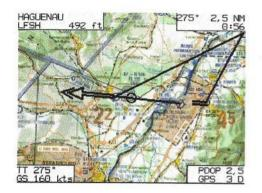
After a flightplan has been activated it is automatically shown as a black line on the map.
