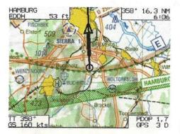
If the flight direction arrow and the Direct to - line are pointing in the same direction, the aircraft is on a direct path to the navigation point (waypoint). The small delta arrow is no longer visible.
