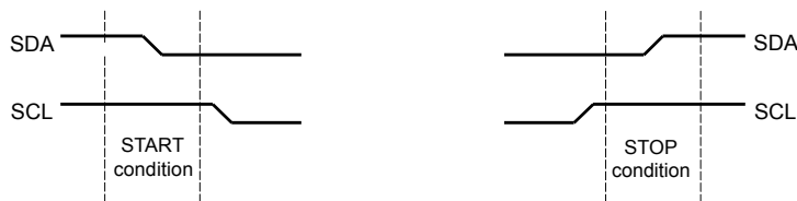
Figure 21-3. START and STOP Conditions
